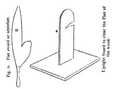
the breadth of this knife is important; when too narrow it easily causes the Flax to twist round it, and thereby tears a portion of the fibres. With this knife the Flax is repeatedly struck, parallel to the board (and close to the slit), with perpendicular blows, to scrape off its wooden asperities. The part which lies in the slit is continually changed by a motion of the left hand.
